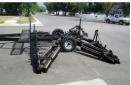
innovative method uses a "scrub" broom system that effectively fills pavement cracks and voids, rejuvenates the pavement, and reduces chip loss. A scrub seal is a good option for roadways that are in relatively good condition with some cracking and without rutting or pavement failures. The expected lifespan of the product is four to eight years.
